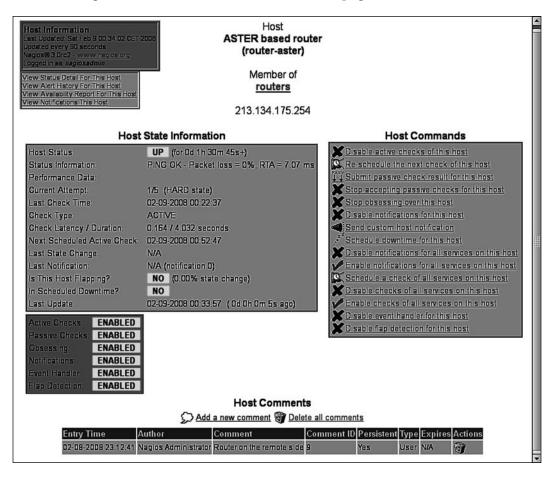
This page contains detailed information of the selected host. It shows the current status and the host checks that have been, or will be, performed. It also contains information on which functionality is enabled or disabled for specified host, whether the host is flapping along with flapping threshold value.
