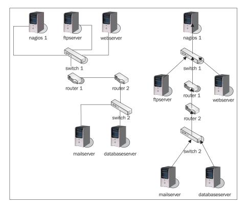
The actual network topology is shown on the left, and the parent hosts setup for the machines is shown on the right. Each arrow represents a mapping from a host to a parent host. There is no need to define a parent for hosts that are directly on the network with your Nagios server. So in this case, switch1 should not have a parent host defined.
