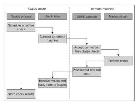
Nagios determines that an active check should be performed. It runs the check\_nrpe plugin that connects to the remote host's NRPE daemon. After the NRPE daemon accepts this as a valid host to send commands to, check\_nrpe sends the command to be run along with any parameter to the remote machine.
